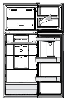
Although this appliance automatically defrosts, a layer of frost may occur on the freezer compartment's interior walls if the freezer door is opened frequently or kept open too long. If the frost is too thick, choose a time when the freezer is nearly empty and proceed as follow:
